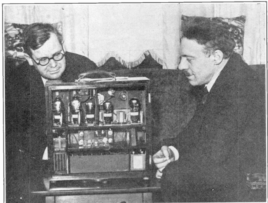
Portable receiving sets are all the rage in Europe. Here is the latest set, built by the Rees-Mace Company with factories in England and France. It uses two screen-grid tubes. This set is now on the American market, having been introduced by John Wanamaker's of New York City. It is entirely self-contained with a special kind of speaker and contains a British wet-battery of very compact design and is non-spillable.
