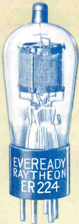
Eveready Raytheon Screen-Grid Tube, ER 224. The size and weight of the elements in this super-sensitive tube make the 4-Pillar, cross-anchored construction absolutely vital to proper tube performance. Without Eveready Raytheon's sturdy construction, the tube is delicate, liable to severe damage in shipment.
