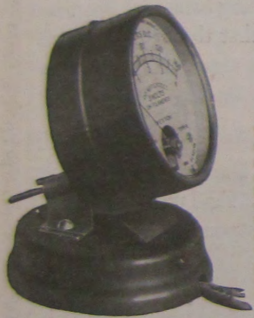
Testing "B" Battery with the Pin-Jack Voltmeter and High Range Stand.
