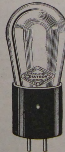
No. 201A Detector or Amplifier (With long prong base) Filament Volts ..... 5 Filament Amps ..... .25 Plate Volts . . . 22 1/2 to 135
