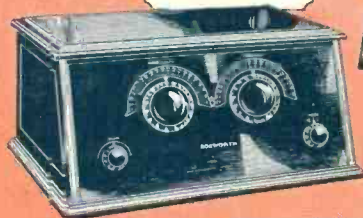
Type B-3 6 tubes, single Control, three stages tuned r-f, detector, two a-f. Price $155.00
