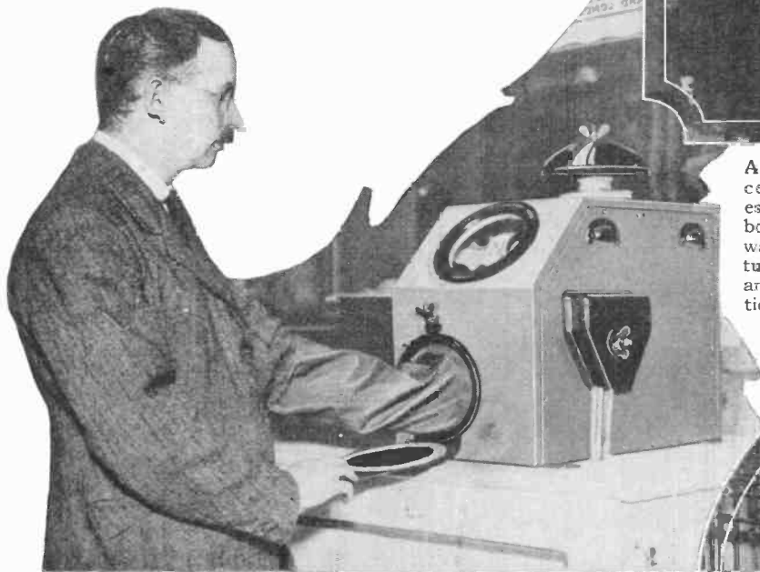
A "shadow-sensitive" vacuum tube is the newest radio invention. Vik Zworykin, of the Westinghouse Company, is shown above with his latest discovery—a radio tube that is actuated by the slightest shadow that crosses it.
