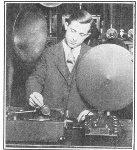
The "Comparaphone," made by the Bristol Company, Waterbury, Conn., permits easy demonstration of three loud speakers, by sending phonograph music through each one in turn, almost instantaneously.
