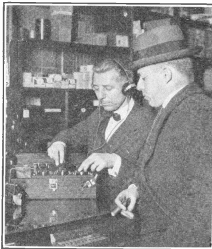
A. W. Mayer of Boston is convinced that testing instruments play a large part in the radio dealer's service facilities. He is shown here testing a fixed condenser. At the head of the page is a view of the Mayer store interior. Note the wall switch at the extreme right, permitting four loud speakers to be demonstrated consecutively.
