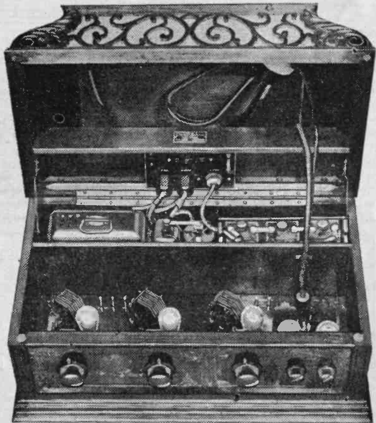
Fig. 1. A Five-Tube Set with Speaker in the Cover. "B" Eliminator and Trickle Battery Charger Are with Battery in Rear.
