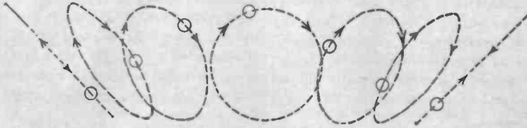
Fig. 11. A Vibration That Starts with a Slant to Left Goes Into a Circle, and Later to a Line Slanting to Right.
