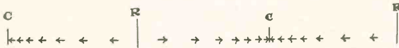
Fig. 3. Air Waves Are Different. The Molecules Crowd Together and Spread Apart Again
