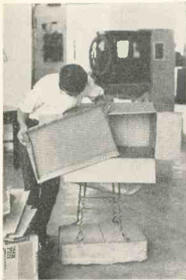
Fig. 2. Assembling the Air Cushion Box
