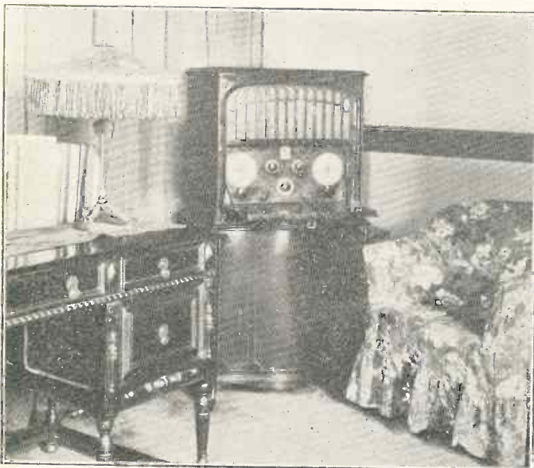
Fig. 4. Even Aerial and Ground Not Needed Here, as Loop is Concealed in Base
