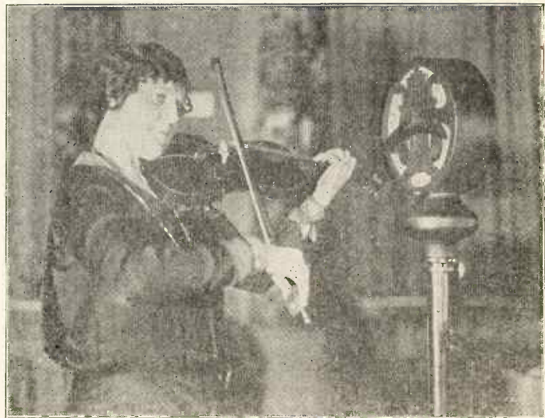
Fig. 4. Harp-and-Spark Microphone at WJZ
