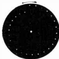
The scanning disc, to show the image in correct arrangement, must revolve in the direction opposite to those of the hands of a clock.
