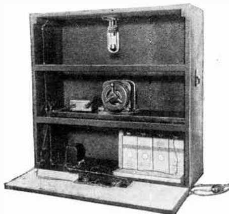
The cabinet of the reproducer with the front removed, showing the lamp and the motor with its regulating condenser. The "B" blocks are conveniently located beneath.
