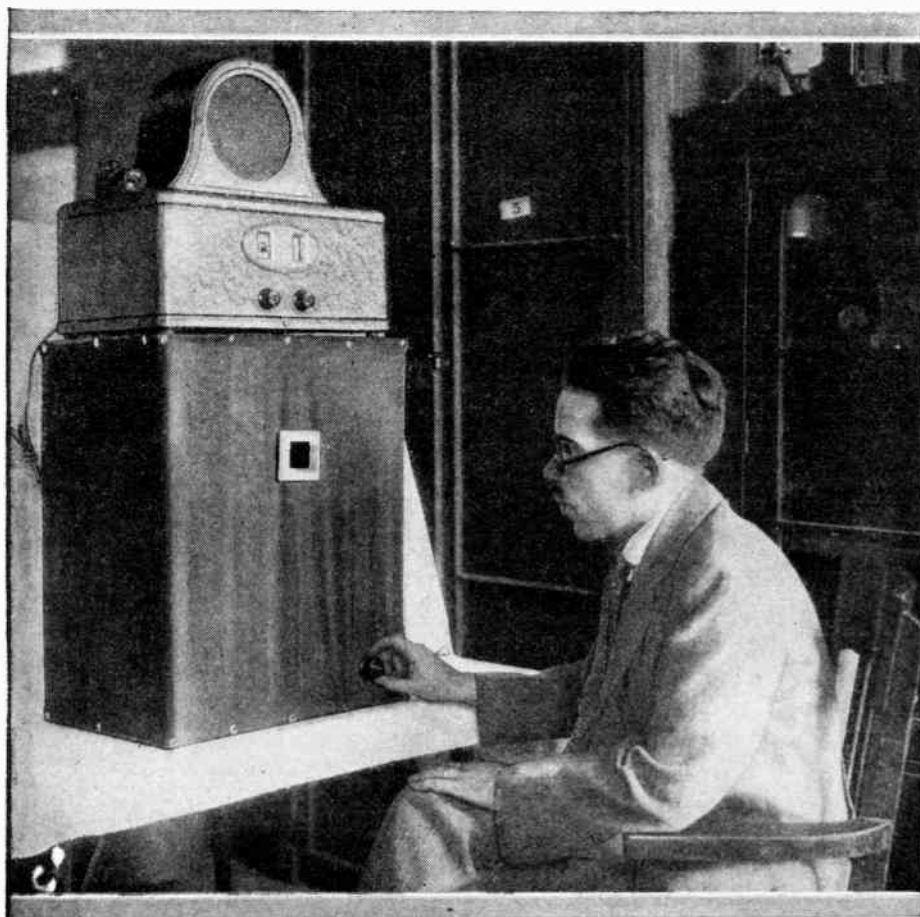
Fig. A. The experimental television receiver in the RADIO NEWS Laboratories. The only adjustment is the knob regulating the motor's speed. The patterns created by the music are observed through the square hole cut in the cloth, opposite the neon lamp.
