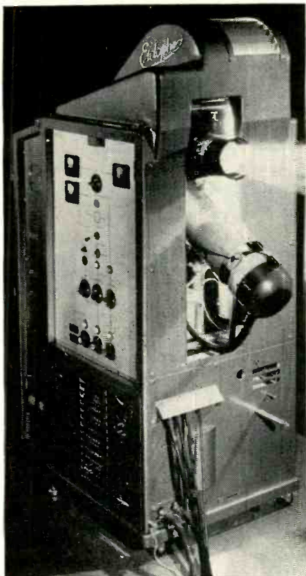
The 5-foot projector weighs 800 pounds; projects a 12 x 16 foot color picture.
