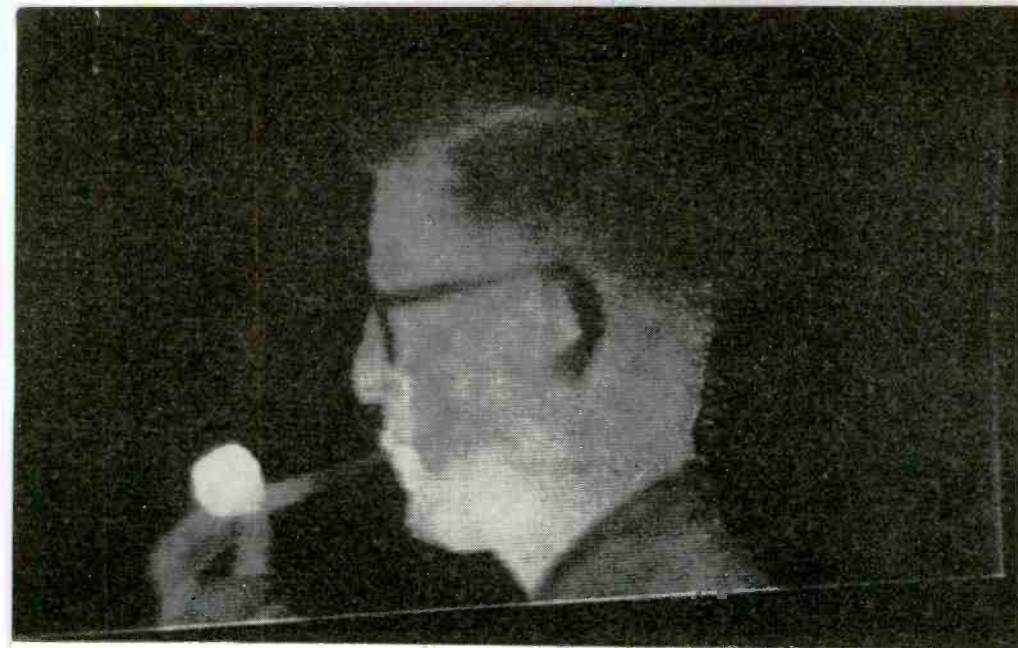
Fig. 1. Infrared photo (thermograph) taken in total darkness. In this view black areas are at a temperature of 75 degrees F or colder, and white areas are at 133 degrees or hotter. Note that the pipe bowl is the hottest object in the photograph.
