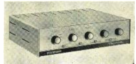
Pacemaker Stereo, shown here, is a low-cost 2-channel 20 watt amplifier. Known as the Model 2221, this Bell product has inputs provided for sterea records, tuner and tape. Plays monoural programs at the flick of a switch.
