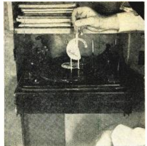
Measuring phonograph stylus pressure.
