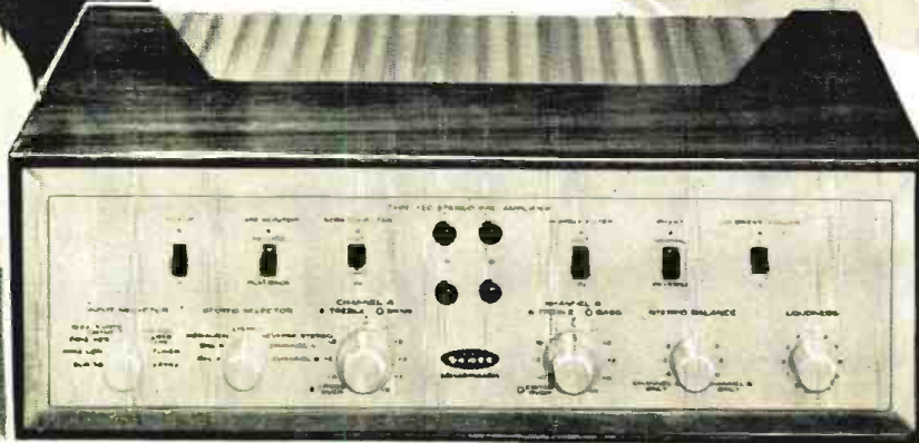
Front panel view of stereo preamp showing arrangement of all the operating controls.
