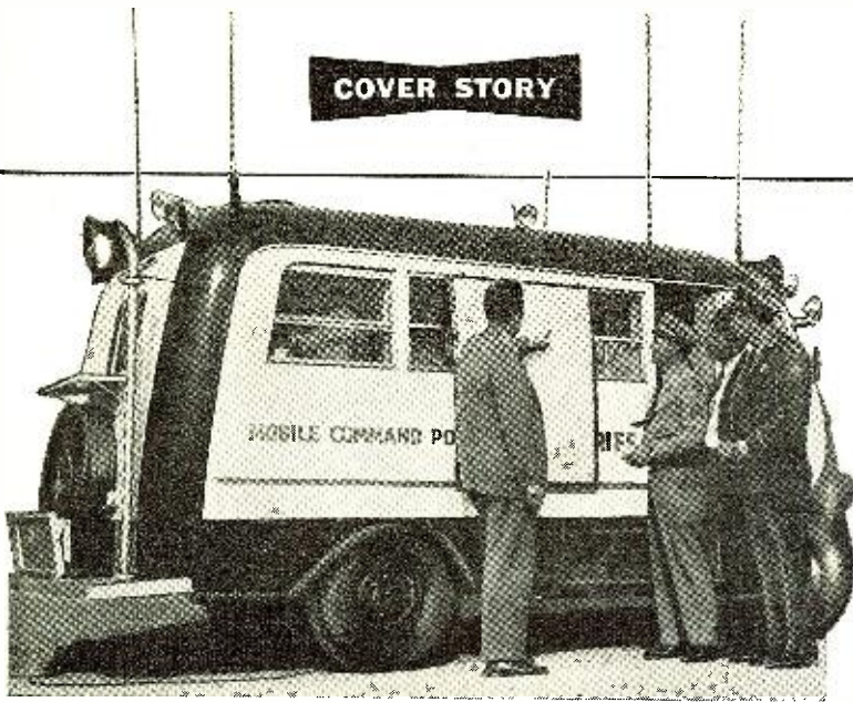
Antennas atop mobile command post truck are for rescue frequencies.
