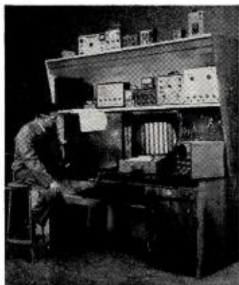
COVER PHOTO: A "service engineered" test bench, designed by General Electric, speeds servicing by improving efficiency of shop. See plans for building bench on page 51 and suggestions on selecting test equipment, page 45. (Ektachrome by Burns Photography Inc.)
