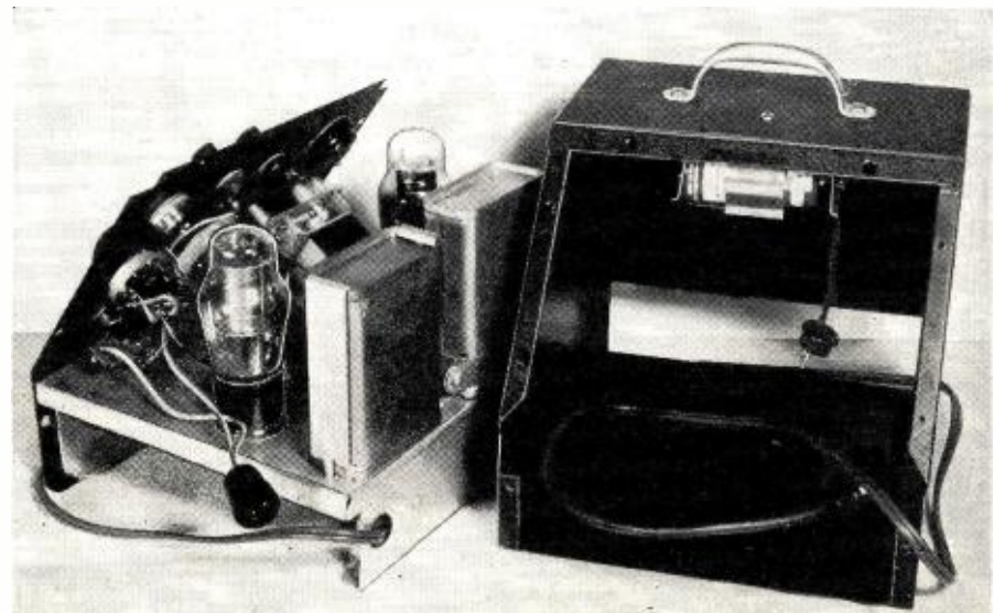
Fig. 3. Unit removed from cabinet, showing mounted battery and connecting cord.
