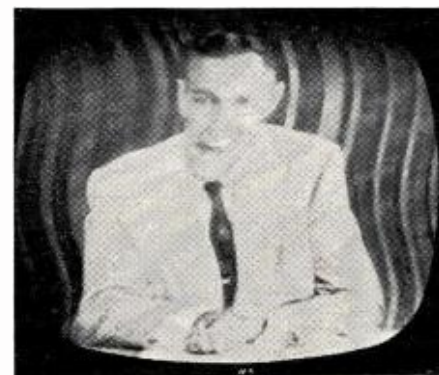
Fig. 4. An open .005- \mu fd. capacitor in the filter network at the grid of the oscillator may cause this weave. Under some conditions, the number of cycles of weave will be considerably greater.
