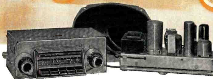
Fig. 1. The "Custom Deluxe Wonder-Bar," Model 987577, directly above, features push-button and search tuning, push-pull output, printed wiring, and a separate subchassis for power supply and audio output. Model 987575 (upper right) uses low-plate-potential tubes and transistor output. Model 987573 (lower right) is a standard tube-vibrator unit.
