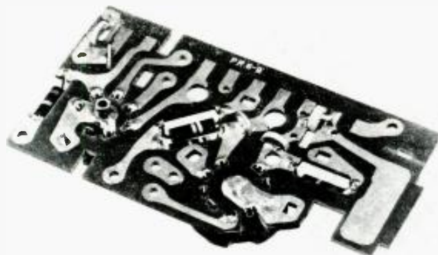
Fig. 3. Shown here is the printed-circuit board used in the new TV tuner. All components and tube sockets have already been assembled on the board. The rectangular conductor area on the right is part of fine tuning mechanism.
