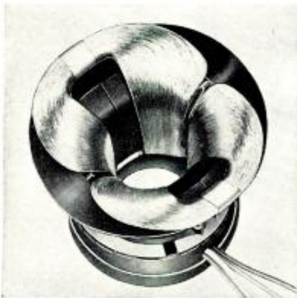
Fig. 3. Typical 90-degree deflection yoke used with 90-degree deflection angle picture tubes. Notice the wide flare of the yoke's horizontal windings.
