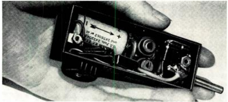
Fig. 3. Top view of the "Injecto-cal" showing the location of parts and compactness.
