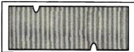
Fig. 5. Theoretical waveform at output from high-pass filter in intermodulation meter. The following demodulator and low-pass filter to remove the "carrier" will not be capable of faithfully measuring this envelope.
