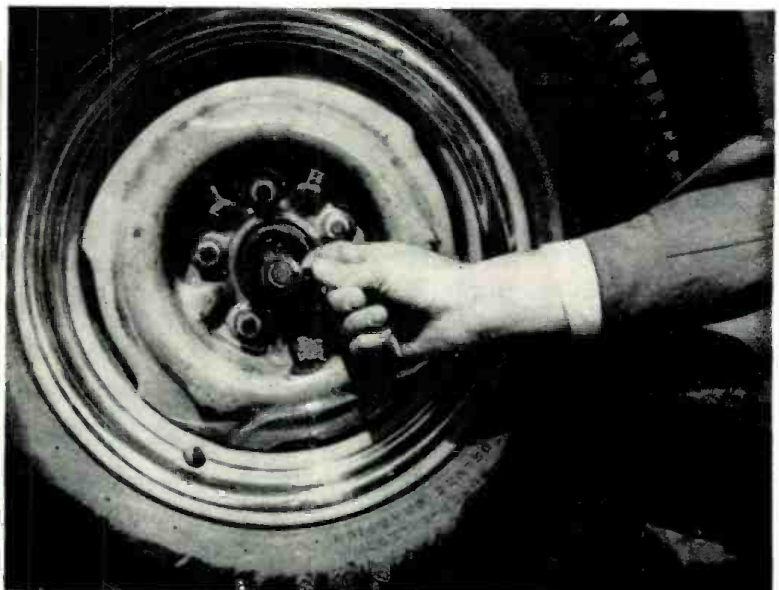
Fig. 5. To eliminate "front wheel static," place a spring made for this purpose under the grease cap on the front wheel.
