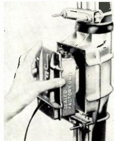
Fig. 12. Some rotators have an easily removable motor and gear train assembly as shown here. The units are factory sealed and usually "lifetime" lubricated.
