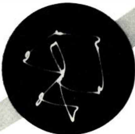
Fig. 8. Vector phase display obtained on an oscilloscope connected to a color TV set. A color-bar generator furnishes the input to the set. See text.
