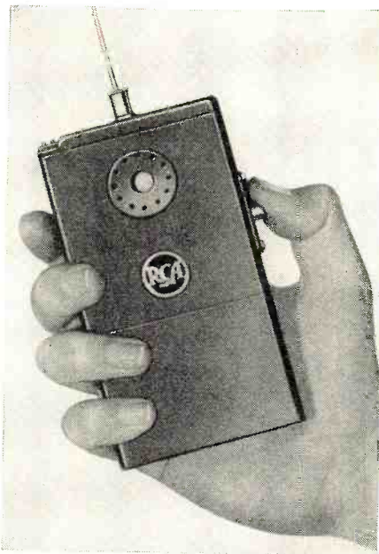
The newly-developed RCA ultraminiature FM transceiver which operates on frequencies between 45 and 50 mc. and utilizes 12 transistors. It weighs 15 oz. Range is 1/4 mile.
