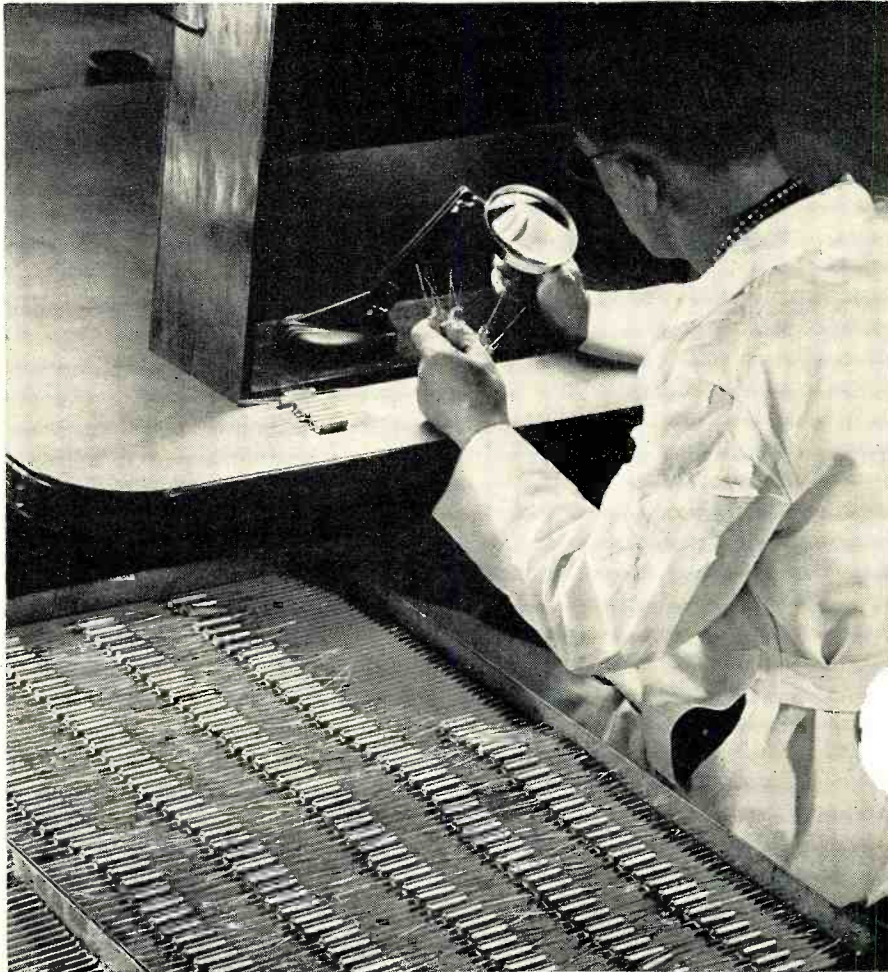
Oil-filled capacitors are subject to vacuum under elevated temperatures, then are individually examined to insure complete hermetic seal.
