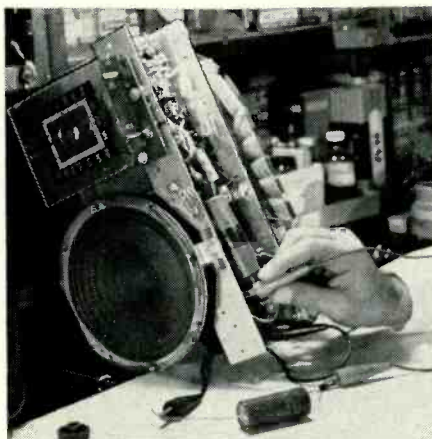
Fig. 4. Shunting a filter capacitor with the 8- \mu f. electrolytic testing unit. To check for a shorted capacitor, disconnect one of the terminals of the suspect.
