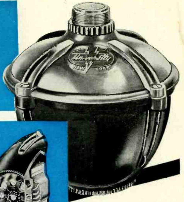
Over-all view of the University driver unit with a close-up of the wattage input steps for 70.7 constant-voltage line and the corresponding impedances for these wattage steps as seen by the amplifier used in system.
