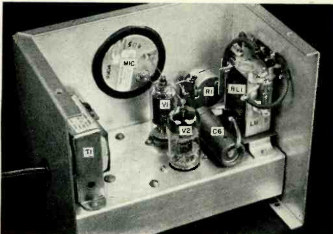
Fig. 4. Top chassis view with various parts identified.
