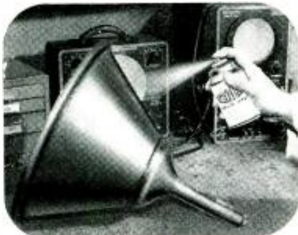
Spray tube bells with Krylon Crystal-Clear or Flat Black to minimize chance of arcing.
