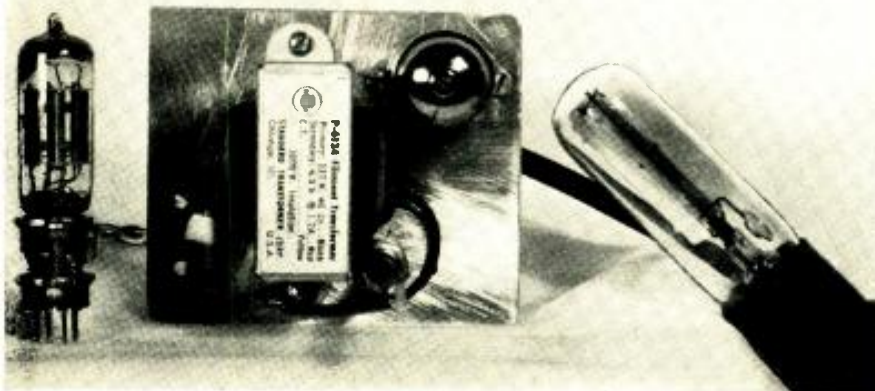
Fig. 4. Complete photoelectric contrast control. The socket adapter for the video amplifier is at left. The phototube must be exposed to room lighting.
