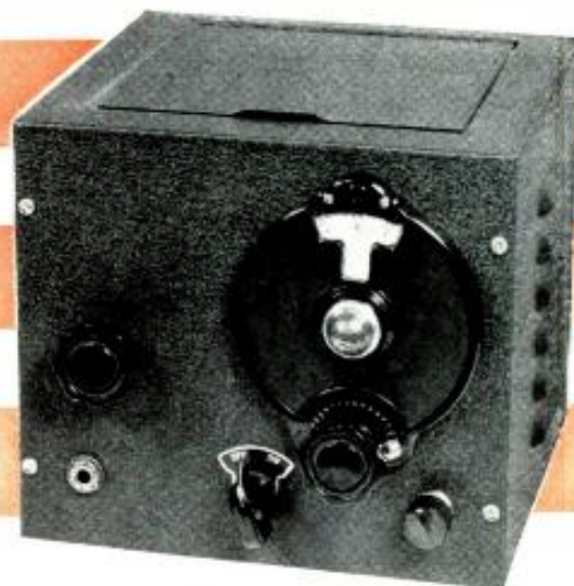
Over-all view of the home-built regenerative short-wave receiver. It is housed in a cabinet which measures 8 x 8 x 7 inches.
