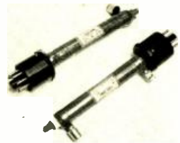
Fig. 3 A dummy pair of horizontal output tubes, for replacement of the 6BG6 output tubes during sweep tests of chroma circuits. Dummy tubes maintain normal load on the receiver power supply for proper d-c distribution.
