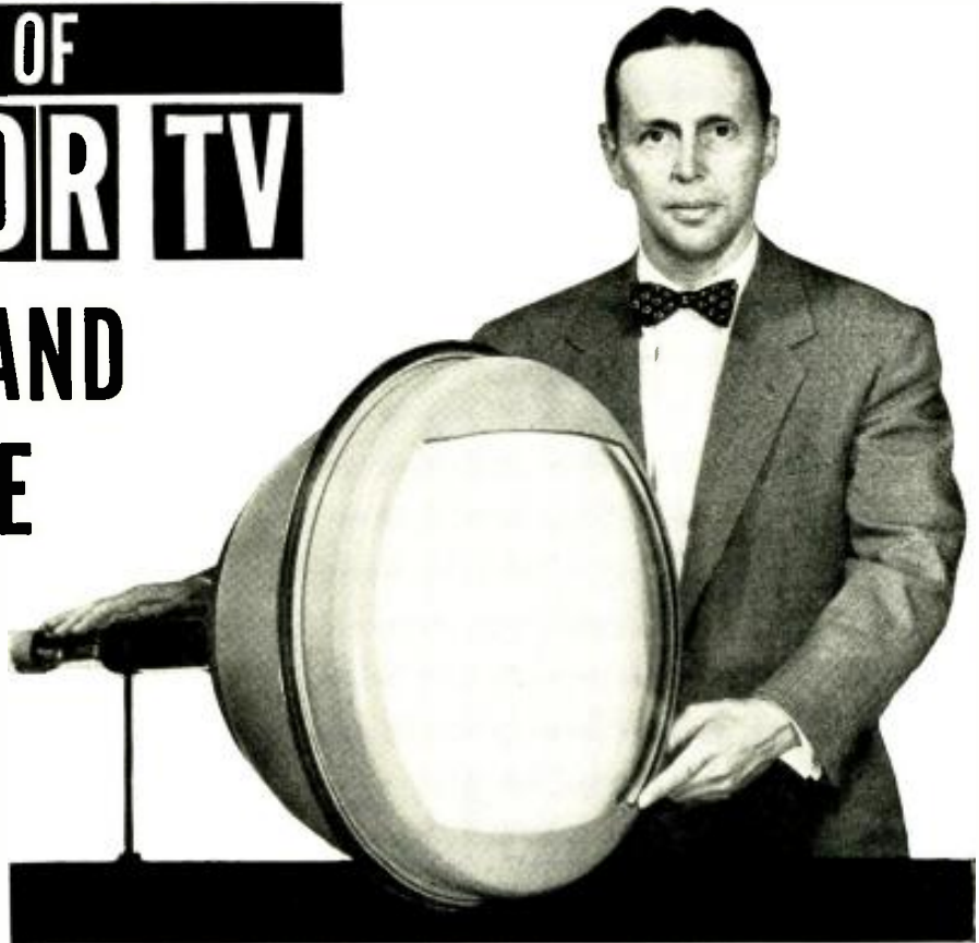
The new CBS-Hytron 19-inch color TV picture tube. This type 19VP22 tube uses three guns and a curved shadow mask with the phosphor-dot pattern on the curved face plate.
