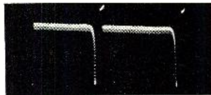
Fig. 4. Oscilloscope waveform obtained at the video output with the switch in position 3 furnishing the grid pattern.
