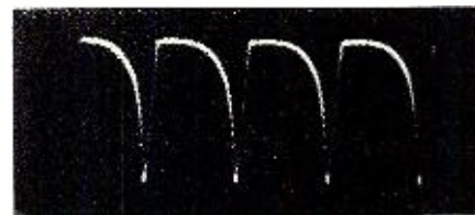
Fig. 5. With the selector switch in position 4 the output waveform shows a sharp spike for each vertical bar.
