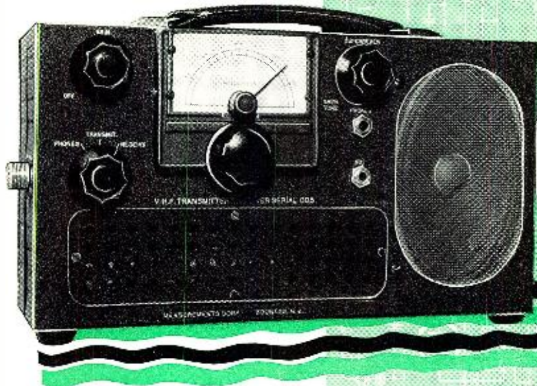
Fig. 1. Panel view of the 146 mc. transmitter-receiver which is built in a compact, portable case. The various panel controls are identified in the text.
