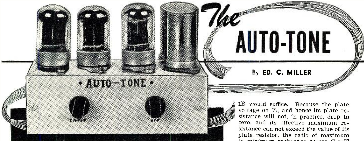
Front panel view of the "Auto-Tone." Three 7F7's are used although almost any twin-triode can be substituted if desired.
