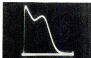
↓ Fig. 2. A typical video response to a square-wave input; notice the poor low-frequency response of this video circuit.
