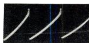
↑ Fig. 4. Sweep circuits can be checked for voltage and current waveforms by means of a wide-band oscilloscope and test probes. Shown here is the deflection coil current of a conventional television receiver circuit.
