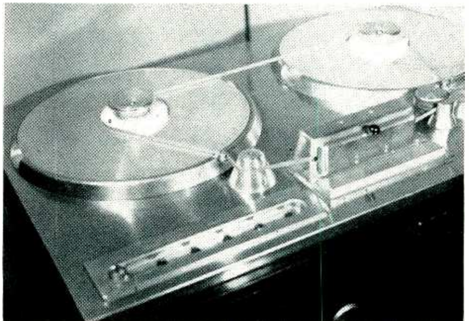
Fig. 3. Continuous tape loop permits reproduction of background sound effects for much longer periods than heretofore available on ten-inch recorded discs.
