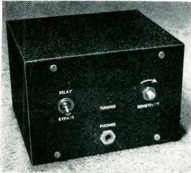
Fig. 4. Front panel view of receiver. Note slot for the screwdriver adjustment cut in shaft of the control, R.
