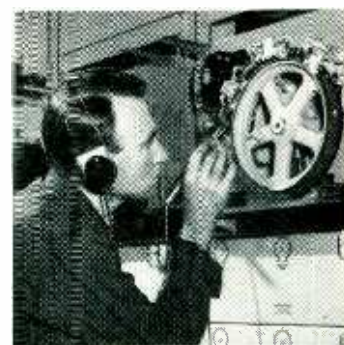
One of a bank of recorder-reproducers operated by the New York Telephone Company for the New York Stock Exchange. They give instant stock quotations to brokers who dial a code number. Recording and pickup heads are shown above wheel.
