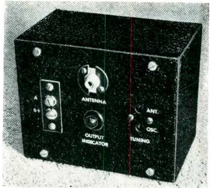
Fig. 5. Over-all view of the transmitter. It is built in a 5" x 3" x 4" box and occupies little space in the car.
