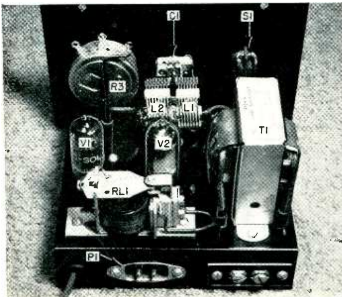
Fig. 2. Rear view of the receiver unit with the major components identified. Over-all dimensions are 6" x 5" x 4".
