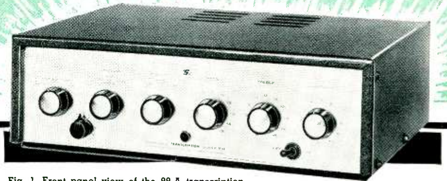
Fig. 1. Front panel view of the 99-A transcription amplifier. This 10-watt unit is self-contained.
