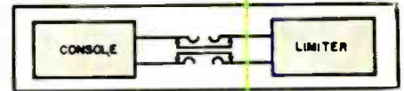
Fig. 4. "Normal-through" jack connection often used in b.c. operations. No patch-cords are needed for ordinary operation as components are connected together through auxiliary or "normal" contacts on jacks. Inserting a cord in either jack removes the associated component from circuit and makes it available on cord for testing or emergency reconnection. The system works equally well with either single or double-type jack assemblies.
