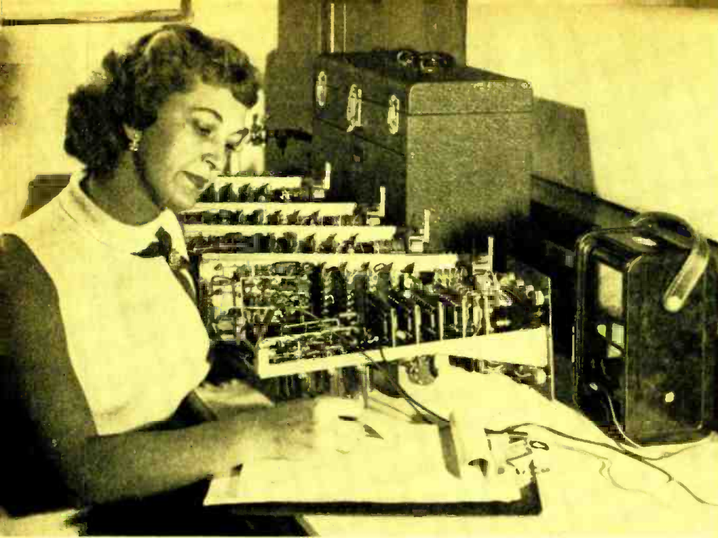
Gate units incorporating the filter sections set up for preliminary inspection.
