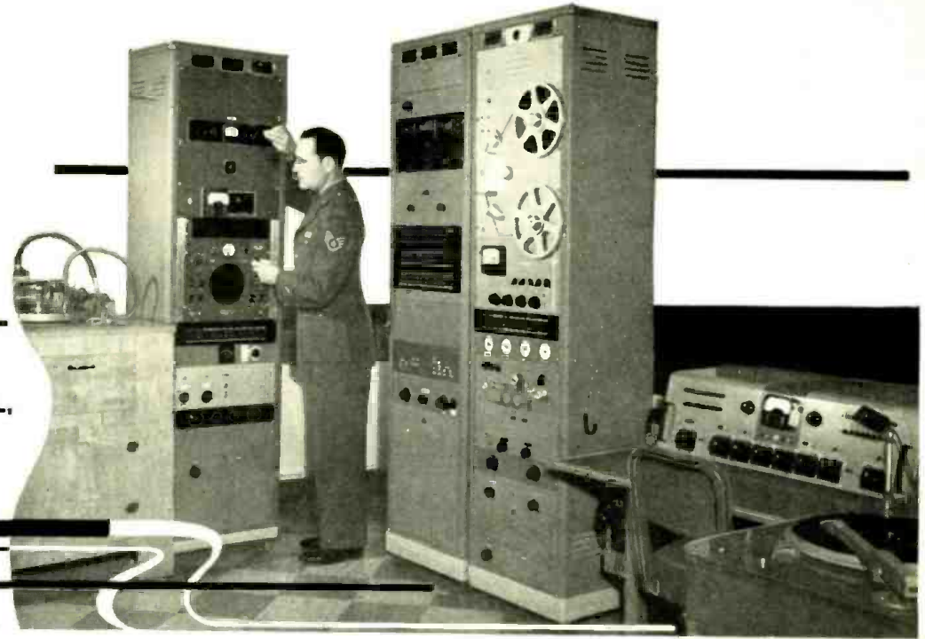
Fig. 1. AFIS control room "A". Rack 1 next to cutting lathes contains limiter and disc recording facilities. Rack 2 includes most of the rack-mounted elements common to both disc and tape channels. Rack 3 carries the tape recorder and also the reverberation generator and the sound-effects filter. These last two items are so located in order to make their panel controls easily accessible to the operator at adjacent console. Staff Sgt. Joseph A. Keddie, chief technician, adjusts levels.
