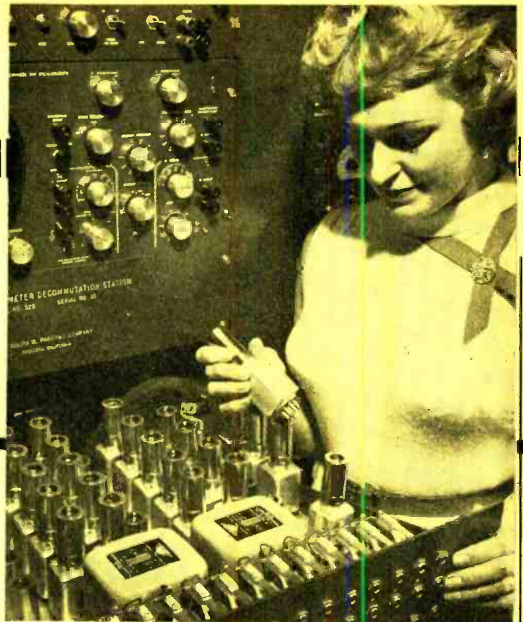
Use of plug-in components, shown above in the gate-triggering unit, permits rapid servicing.
