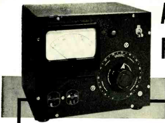
Front and rear views of the home-built unit for monitoring line voltage in the ham shack, service shop, or test bench.
