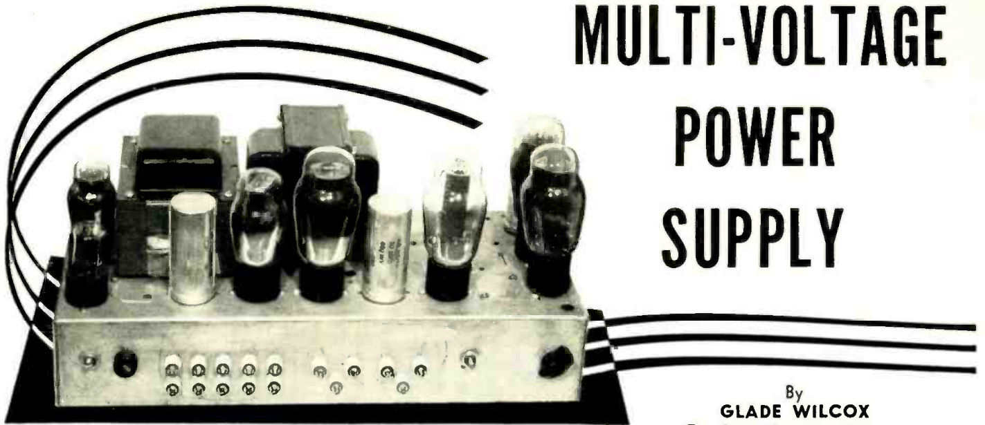
Fig. 1. Over-all view of laboratory-type power supply. It is built on a single chassis measuring 7" x 17" x 3". It uses Thordarson-Meissner T26R00 transformer.
