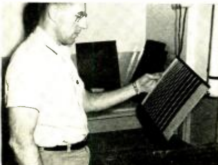
Herman Hausle holds plate which was etched with straight lines for test purposes. Etching machine contains a ferric chloride solution which eats away copper not protected by photographic image.
