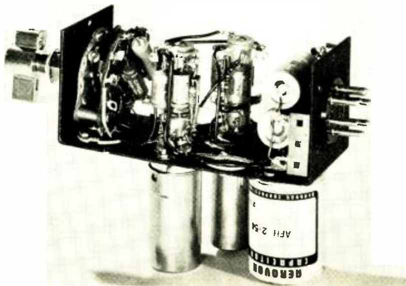
Underchassis view of preamp. Turret socket construction makes unit compact.
