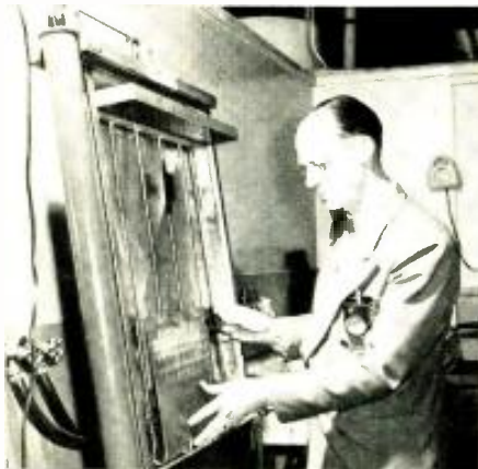
Developing machine contains an alcoholic solution of purple dye, called "cold-top" enamel developing solution. Here John McMaster, chief of the photo template unit, places a plate on the rack prior to lowering it into solution. The plate has a photographic image imprinted on surface.
