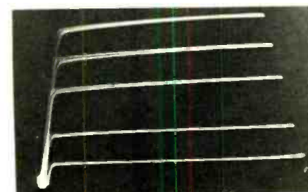
Fig. 5. Family of collector current vs collector voltage curves for Raytheon CK722 at base currents of 25, 50, 100, 150, and 200 microamperes respectively (bottom to top).
