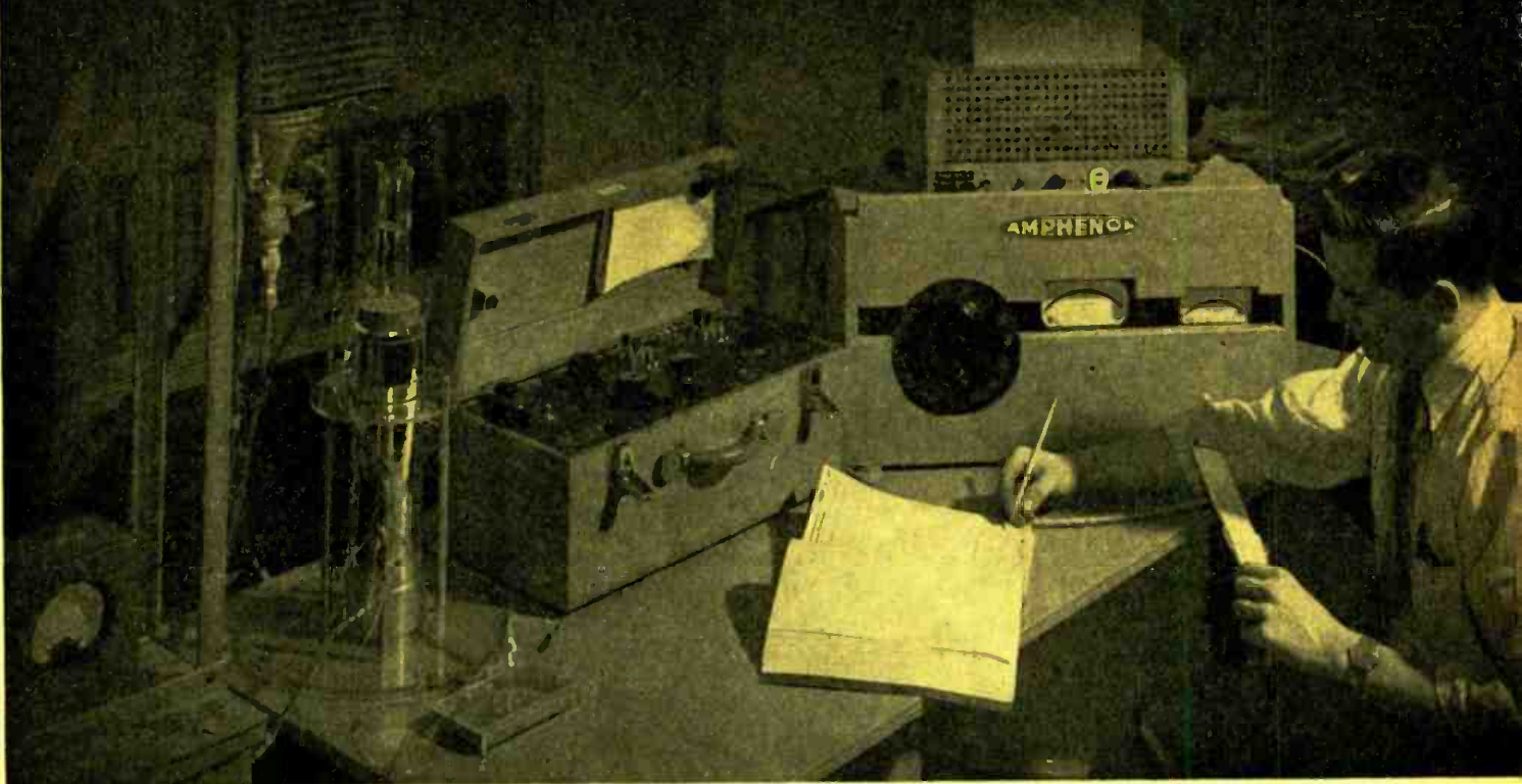
Setup for calorimetric calibration of water load and for making r.f. power measurements.
