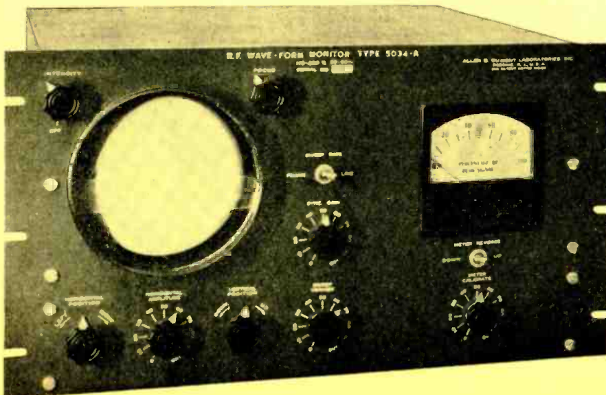
Fig. 2. Waveform monitor for measuring significant amplitude levels.
