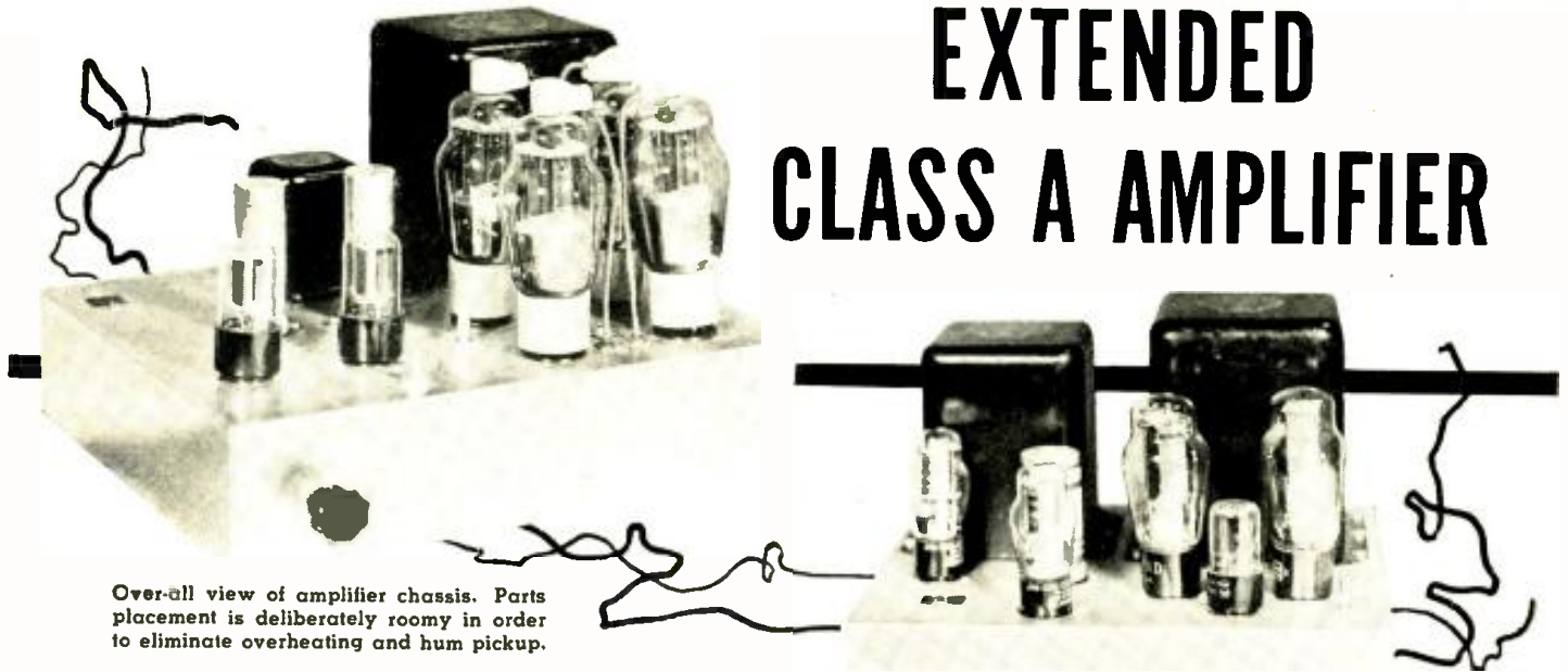
The power supply chassis measures 10" x 12" x 3" and is separate from amplifier.
