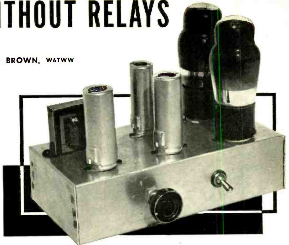
The all-electronic break-in system is small and is easily adapted to most stations using voice control. Well-filtered negative power supply is needed.
