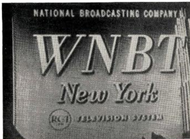
Fig. 3. "Spook" interference with signal of normal strength.
