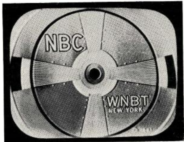
Fig. 5. Effects of regeneration on a test pattern. Note intensification of different parts of vertical wedges (left) and intensification of blacks in bulls-eye region and in lettering and the whites trailing blacks as shown at right.
