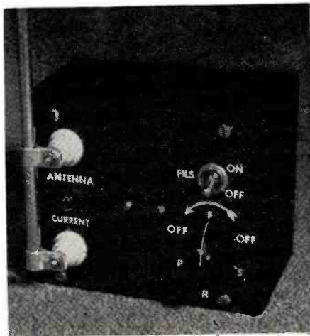
Fig. 2. The 27-mc. "Citizens Band" transmitter, built in a 3"x4"x5" utility box. The batteries are also housed in this box.
