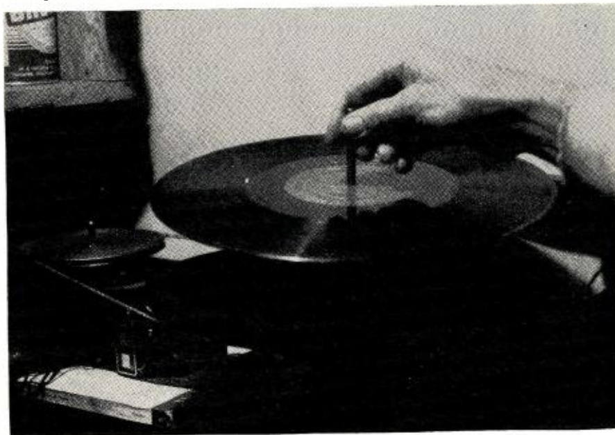
Fig. 5. A long, removable peg with a shoulder facilitates the changing of records.
