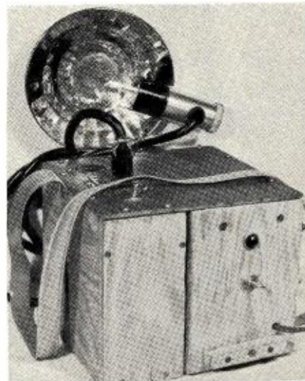
Fig. 4. Over-all view of complete unit. The cabinet measures 7"x6 1/8"x6 3/4". The 450-volt battery pack weighs 8 1/2 pounds and will provide approximately 1500 flashes.
