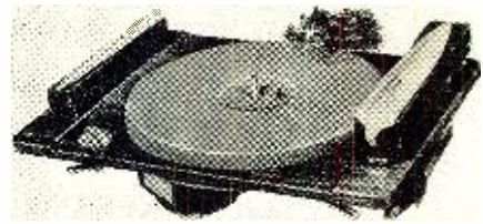
Fig. 2. The General Industries' Model R-85L cutting assembly, showing playback arm at left and recording arm at right. Weighted turntable has retractable drive pin, near center post, to prevent slipping of disc. Speed selector switch is at the left.
