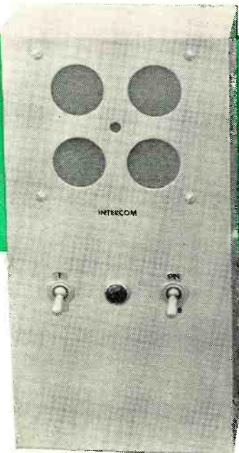
Front view of the master station. Only two simple operating controls are required.
