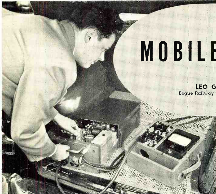
Motorola's "Uni-channel Sensicon Dispatcher," being tested, is operated at the company's Phoenix Radio Service on a 20 kc. channel spacing instead of usual 60 kc.
