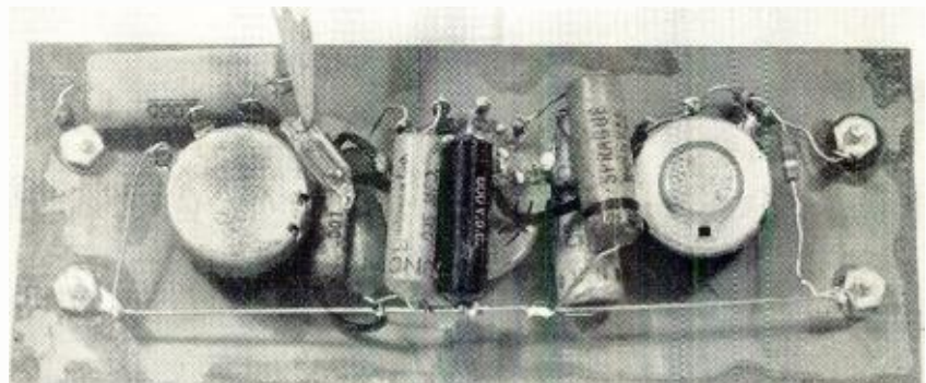
Fig. 4. Rear view of unit. Pencil points to the neon bulb indicator.
