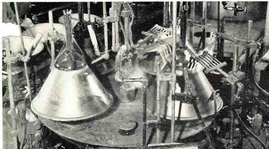
A specially built machine is used to seal the funnel and neck to 19-inch metal cone.
