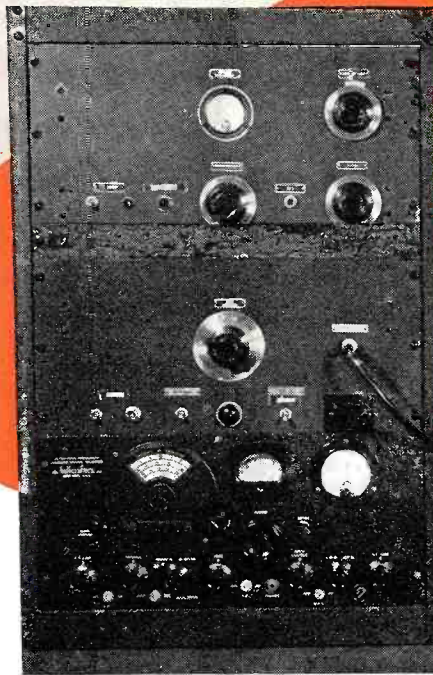
Complete low-power phone station, which occupies a table area of only 14 by 21 inches. Top to bottom: r.f. section, modulator, and Hallicrafters S-36A receiver.
