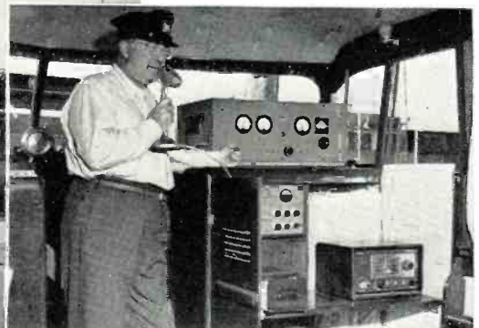
Myron Zobel, W2NMC, aboard the yacht "Norte." With a fixed 10-meter, three-element beam overhead, he has worked all over the world. Equipment is Hallicrafters' HT-18 exciter, HT-3 transmitter, and SX-42 receiver. The three-element beam antenna on the "Norte" excites attention wherever the boat goes. The vertical antennas are for operation on the lower frequencies.
