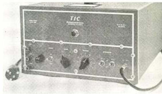
Fig. 4. A sweep oscillator covering the sound and video i.f. frequencies.
