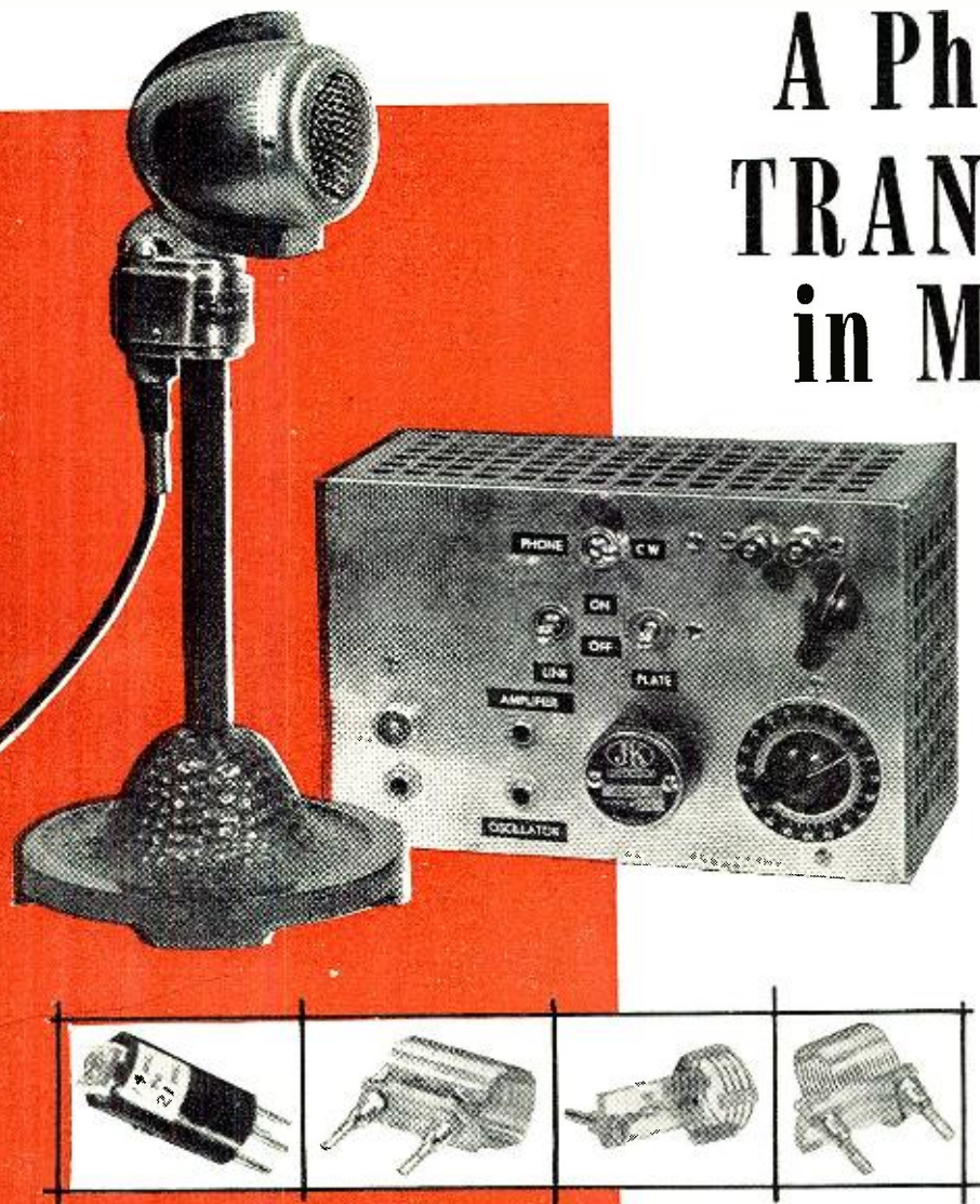
Fig. 1. Over-all view of rig. In front are (from left to right): buffer coil, 80 m. tank coil, 6 m. tank coil, and 20 m. tank coil.
