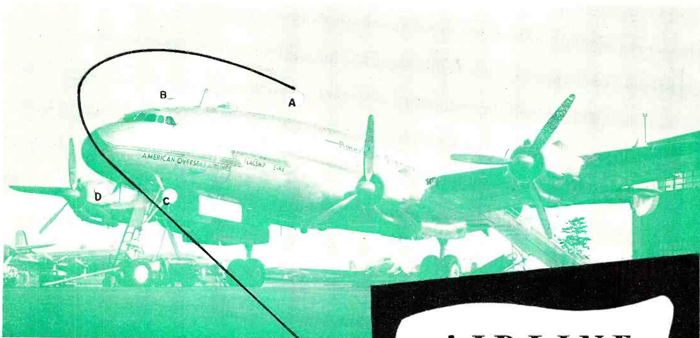
The antennas on this "Constellation" are dwarfed by the plane itself. Shown in the picture are: A, the 77 ft. "V" to outboard stabilizers; B, ILS antenna; C, pilot (air speed indicator) masts which support ends of DF sense antennas; and D, v.h.f. stub.
