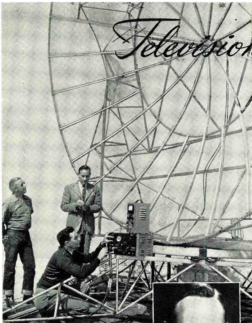
This 16 foot parabolic reflector is located on top of the Mt. Lee television studio. It is used for pick-up of signals from remote locations and is the largest such unit being employed in video work.
