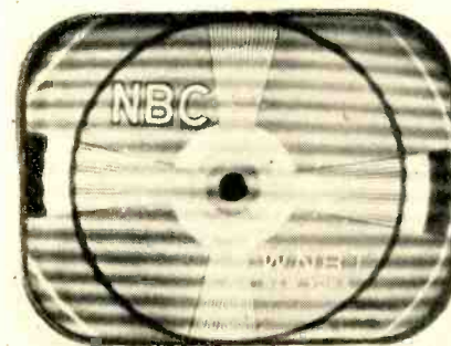
Fig. 6. Bars of varying number and intensity will indicate sound interference.
