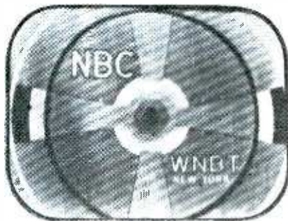
Fig. 8. Beat pattern caused by an interfering r.f. of frequency close to oscillator.
