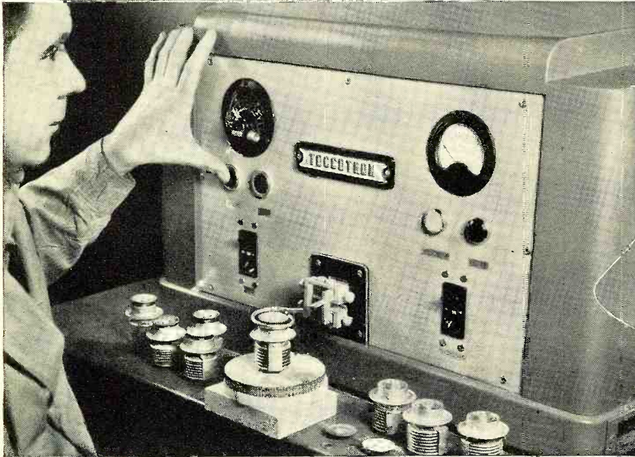
The 750 watt TOCCOTRON, a bench type induction heating machine designed primarily for silver brazing and soldering, but adaptable to other uses.
