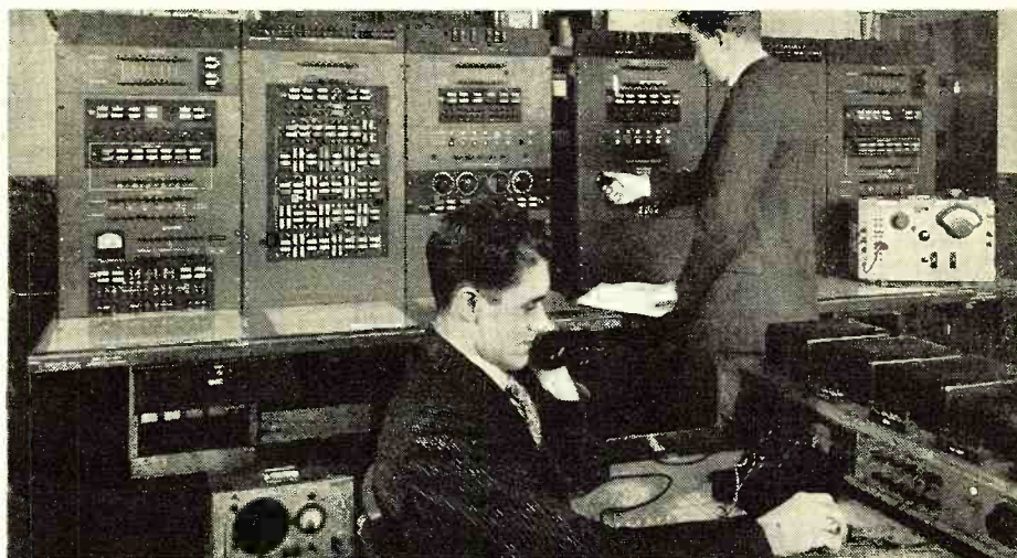
The engineer in the foreground talks over the test circuits which the other engineer sets up on a "circuit simulator."
