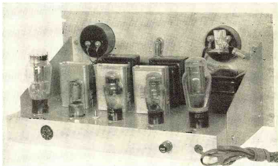
Fig. 4. Rear view of the power supply chassis of unit shown in Fig. 1.
