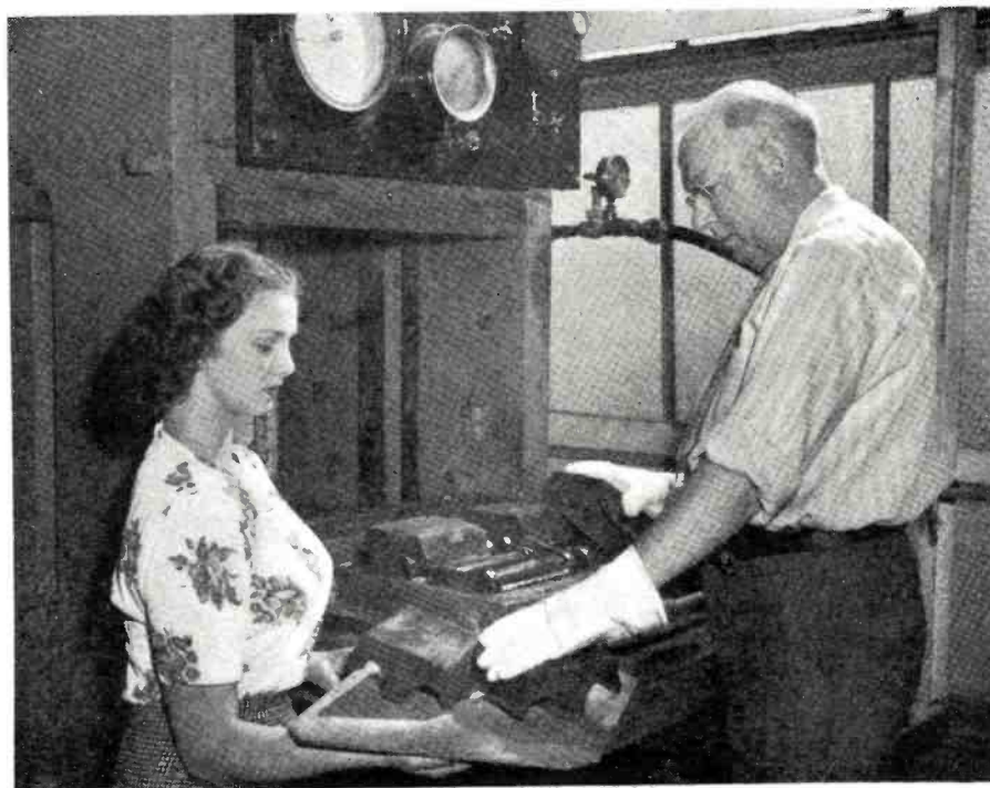
Heat-treated tank tracks are put into this machine and pressed into their metal base. This unit applies steam curing which follows electronic process.
