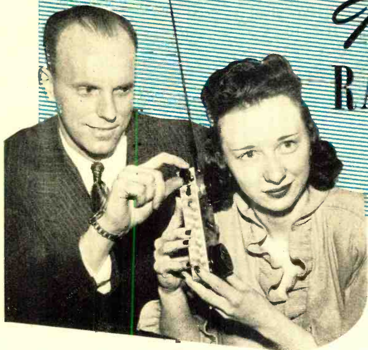
Midget handie-talkie, "Tiny Tim," developed by Charles T. Haist, Jr. of the General Electric Electronics Department. Range of this transmitter-receiver is two miles.
