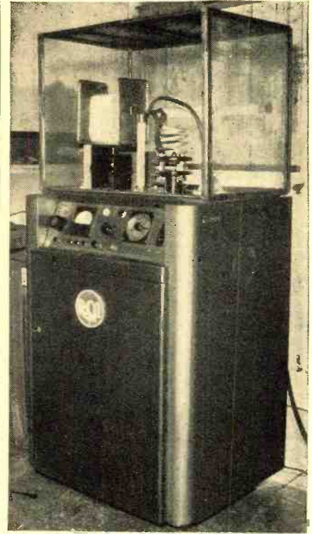
Fig. 5. Experimental equipment that is used to dry nylon yarn on sizing tubes. This process is also used to set the twist of yarns. The time required to dry a sizing tube, containing 800 grams of single-ply, 40-denier yarn with 24 grams water content, is approximately three minutes.
