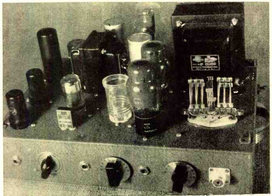
Fig. 3. Top chassis view shows arrangement of components. Parts may be identified by referring to the chassis layout, Fig. 4. 10-meter coils are shown in position.
