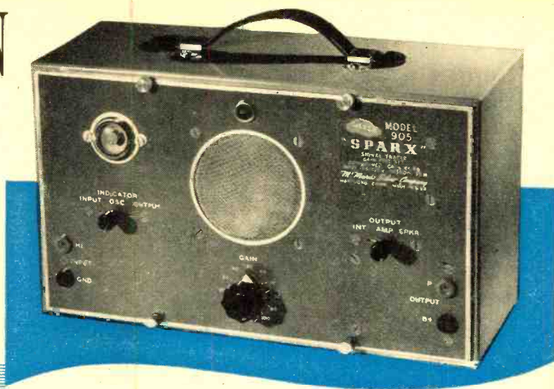
Fig. 1. Front view shows placement of various operating controls.
