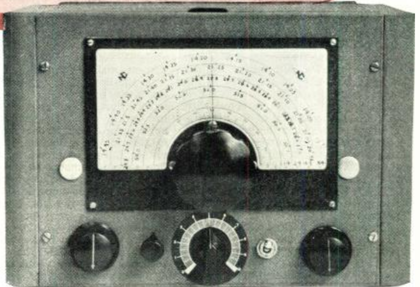
Front panel view of the completed unit. The controls from left to right are antenna changeover switch S_1 , regenerative control R_1 , and S_2 , band set condenser C_3 , filament switch S_3 , and r.f.-mixer condenser C_1 , C_2 . Main knob controls tuning of oscillator condenser C_{12} and superregenerative condenser C_{17} .
