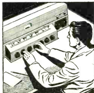
For good reception, program loudness must stay within certain limits. Volume-meters help to hold it there
