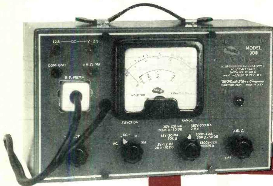
Fig. 1. This new improved v.t.v.m. provides fifty-one total ranges of d.c. and a.c. volts to above 100 mc., ohms through 2000 megohms, current from 1.2 ma. through 12 amperes, db. from -10 through +50.
