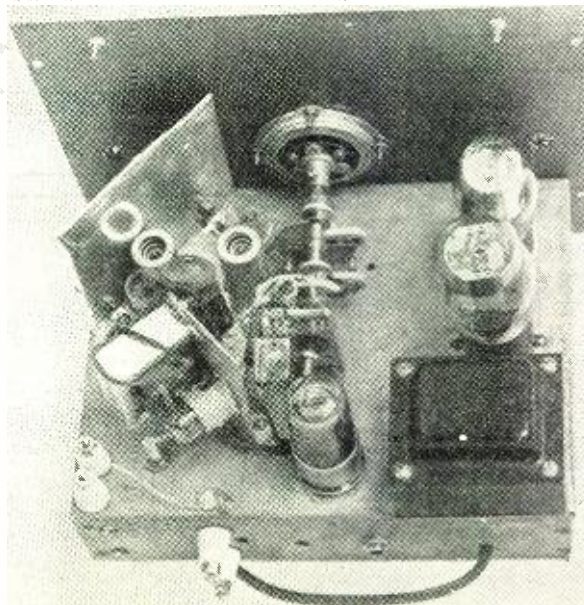
Top view of the completed receiver. The entire assembly is mechanically rigid and all stages are well shielded to prevent any interstage coupling.
