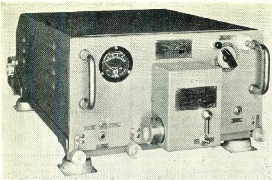
Fig. 5. Illustrating how rubber shock mountings are used on all aircraft receivers.
