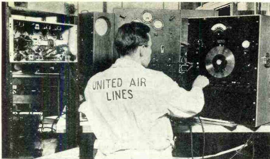
Fig. 7. Test bench set-up in the maintenance shop of one of our major air lines.
