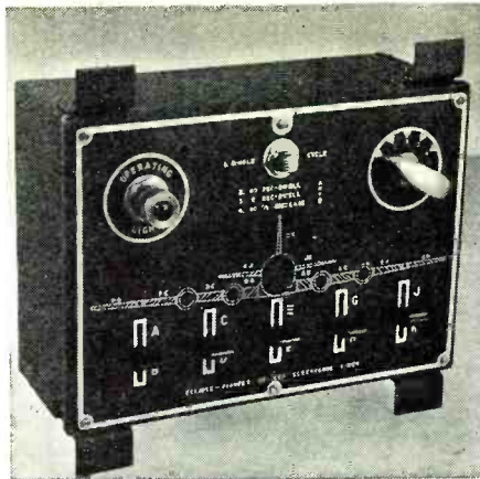
Fig. 4. Typical electronic de-icer timer. This control unit may be adjusted to automatically operate the de-icer boots in cycles, timed to suit various conditions of ice formation and flight altitudes. The de-icer boots are periodically inflated and deflated to break up the ice.
