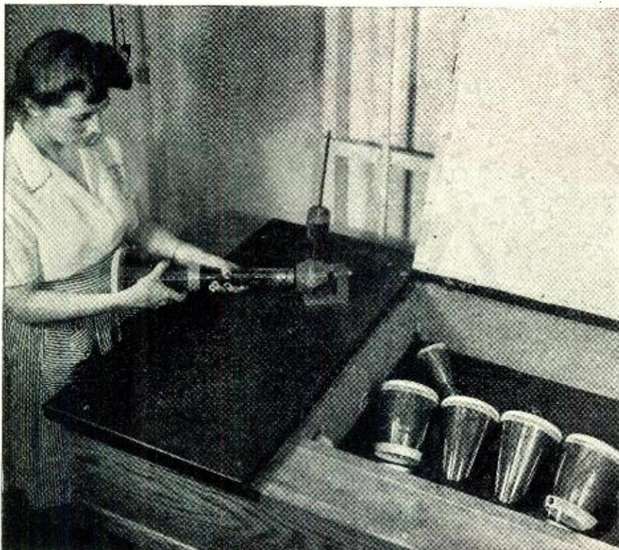
Operator applying the torque test to cathode-ray tubes at the Dobbs Ferry plant of North American Philips Company, Inc. Tubes (lower right) are soaked in warm water for 18 hours—then the base is inserted in the holder and the tube is twisted against the torque of the weight on the arm. This makes sure that the cement holds firm in the base of the tube. Type 5LP1 tube is being tested, while other tubes, shown immersed, include types 5CP1, 5BP1, and 3BP1.
