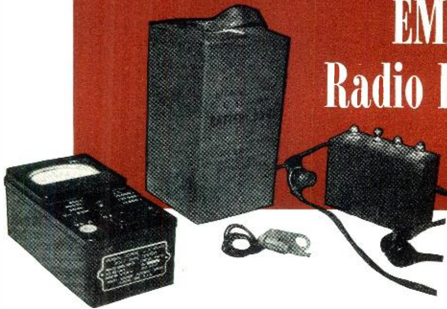
An ohmmeter, neon bulb, and high d.c. voltage source or a small battery and headset, are all that is needed to complete these tests.
