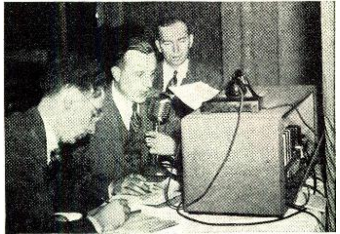
Engineers obtain receiver field-strength reading on the car signals from engineer stationed at the remote receiving end.
