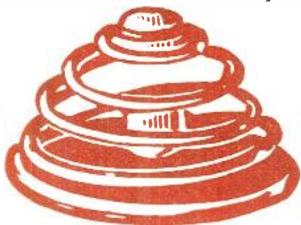
Fig. 2. Coiled spring, mounted directly under hub caps, will suppress wheel interference in the form of static charges.
