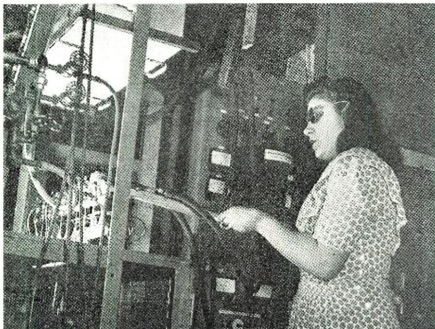
External bombardment of parts in 24G ultra-high-frequency transmitting tube. High-frequency induction heating is used for this work.
