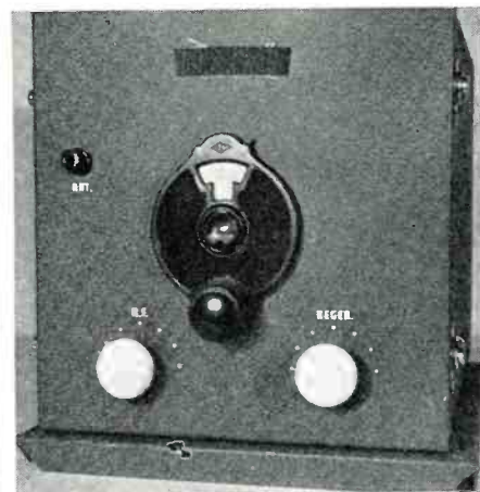
Super-regenerative receiver. Because of their low cost, simplicity and receiving range, the original ones still remain in service even though they squeal to nearby stations and have background hiss.
