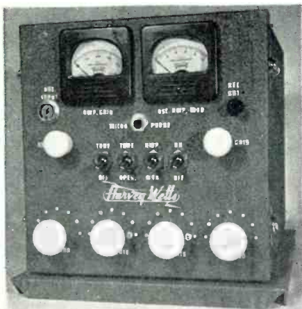
10-watt AM transmitter used by Maine State Police in mobile units.
