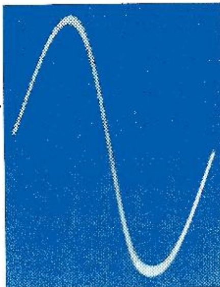
Fig. 5. Sine-wave output obtainable, as pictured at 200 cycles-per-second.
