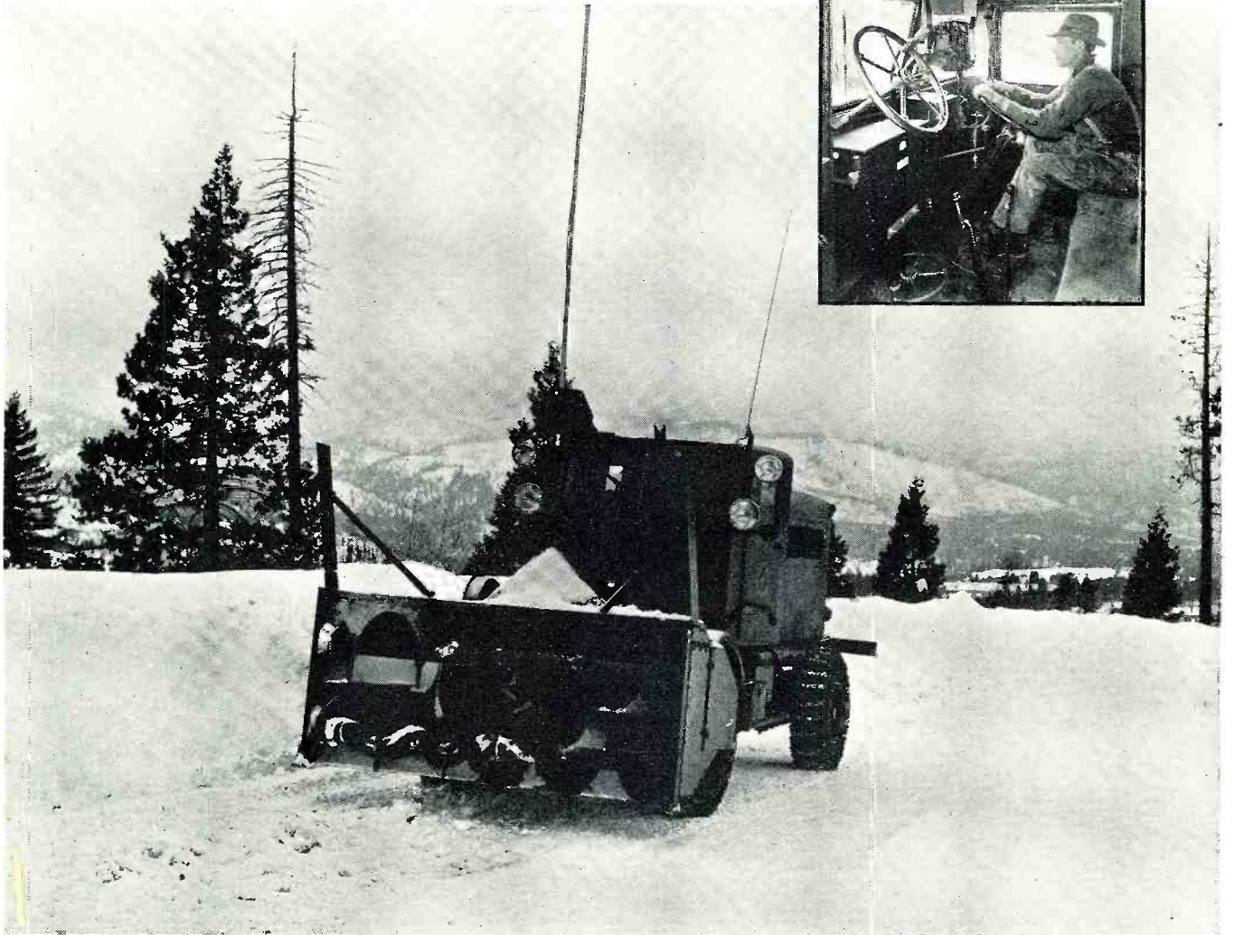
Below: Radio-equipped snow plow with antenna in position. Insert: Plow operator hears instructions from headquarters.
