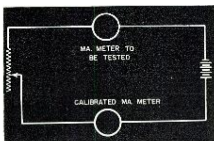
Fig. 1. Calibration setup.
