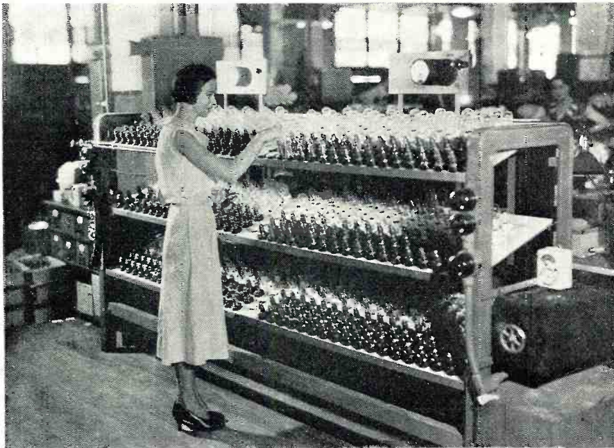
After completed tubes are sealed and exhausted, they are placed in a rack and operated for a time sufficient to stabilize electrical characteristics.
