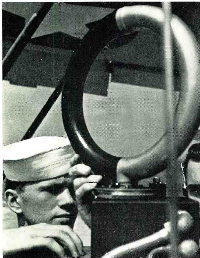
Finding the null point on a signal with a compact shielded loop. Note calibrated scale on base of loop.
