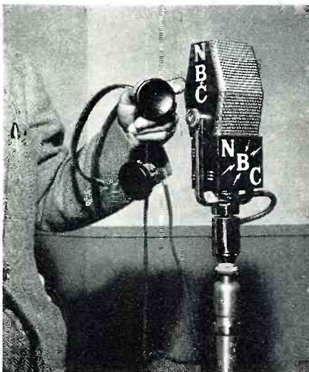
Velocity microphone and earphones used for special sound applications.
