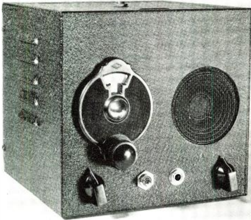
The receiver uses only one tuning and one volume control.
