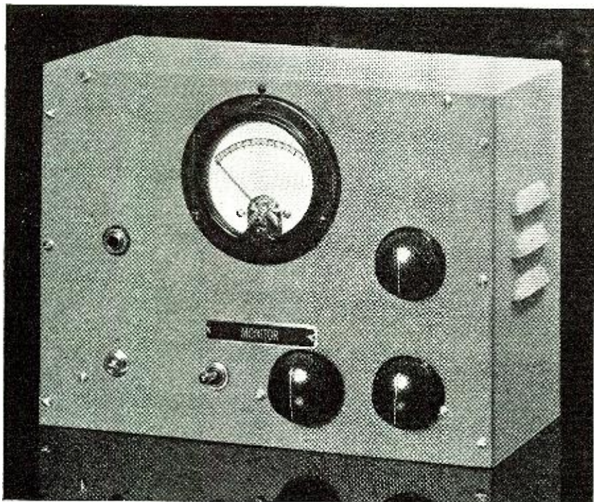
The meter will show any deviation from transmitter frequency.
