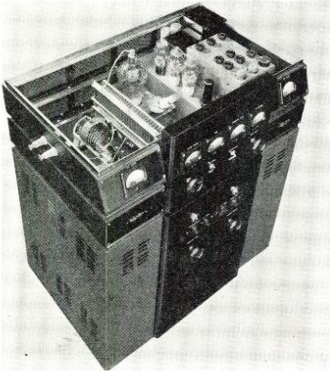
The entire bandswitching mechanism is housed on top.
