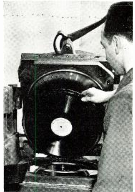
The "master" disk is placed into a press with a "biscuit" and a finished recording is made. A pressure of a ton is used.
