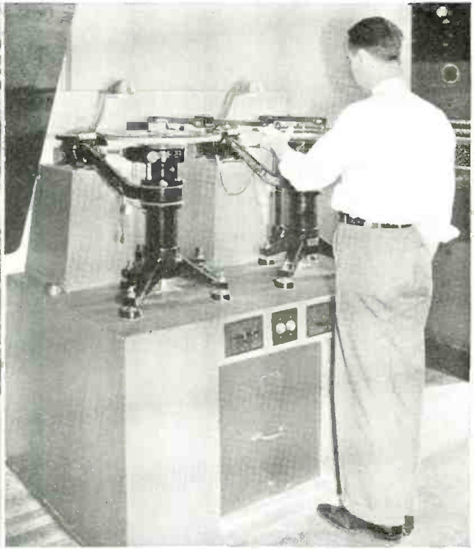
Mounted on a solid block of concrete imbedded in bedrock is the play-back machine for checking the final baked recording.
