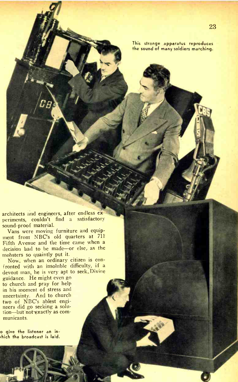
Ray Kelly is holding a box of whistles which, when placed in the wind machine can give forth any tone of wind desired.
