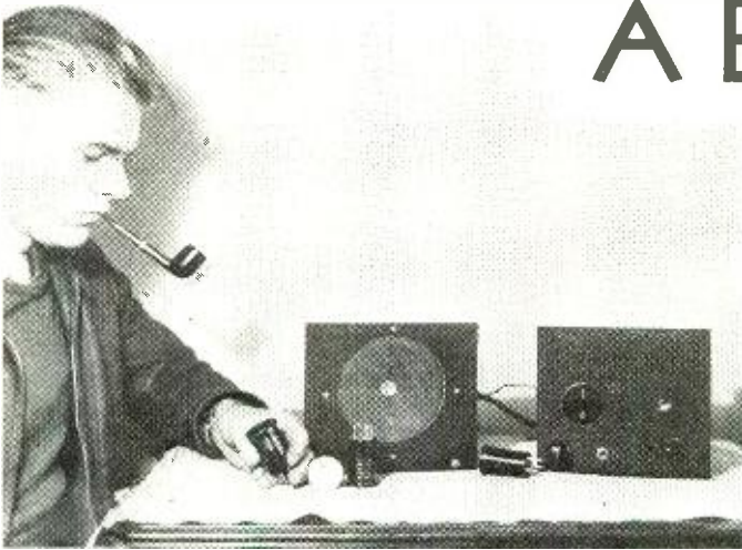
Note two controls on receiver. Speaker is on separate panel to eliminate vibration.
