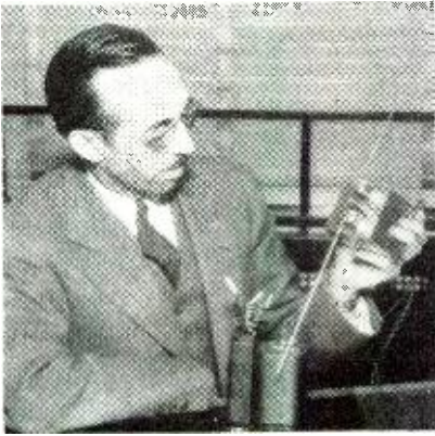
The complete transmitter can be held in one hand. Batteries are used for power.
