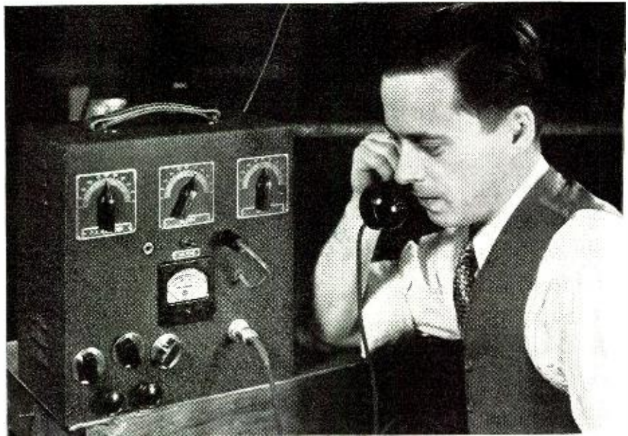
The author tries out the rig. Transmitter on top, and receiver on left bottom. 30 watts of 100% modulated signal on 5 major bands.
