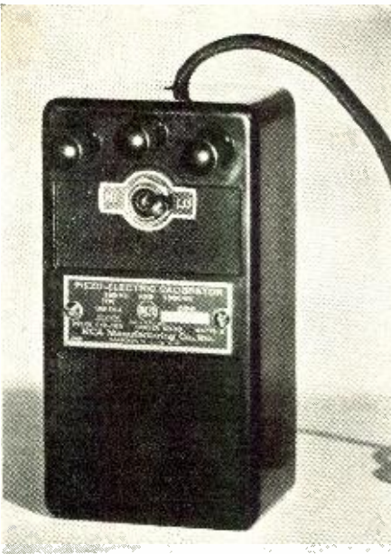
The pre-calibrated crystal oscillator which should be in every serviceman's kit. It has two fundamental frequencies, 100 and 1000 kc.
