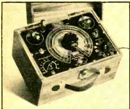
CAPACITOR ANALYZER Figure 3. The Solar capacity meter for measuring condensers and resistors.
