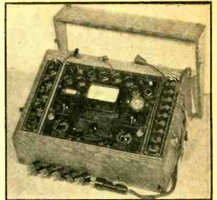
Figure 1. The Triplet tube checker, volt-ohmmeter and output meter.
