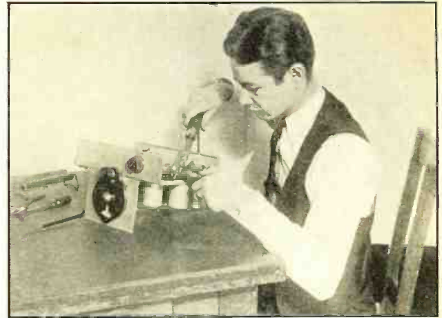
ADDING A.V.C. TO A RECEIVER A half hour's work and the t.r.f. receiver described in Part Nine (last month) of this series is provided with automatic volume (sensitivity) control.
