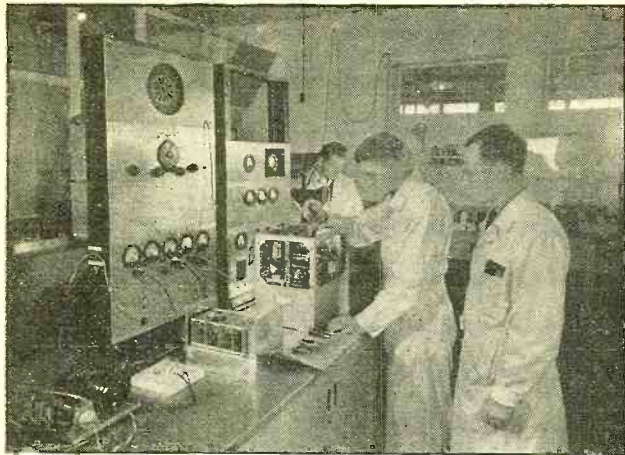
CHECKING OVER AN AIRCRAFT TRANSMITTER A student, under the guidance of an instructor, adjusts a radio transmitter in the shops of the Boeing School of Aeronautics. Test panels are seen in the background and in the foreground is a receiver with its power supply and neon-lamp indicator.
