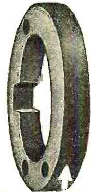
This sturdy molded Bakelite ring supports the carbon resistance element. Arrow indicates flat outer rim to which resistance element is permanently fused.
