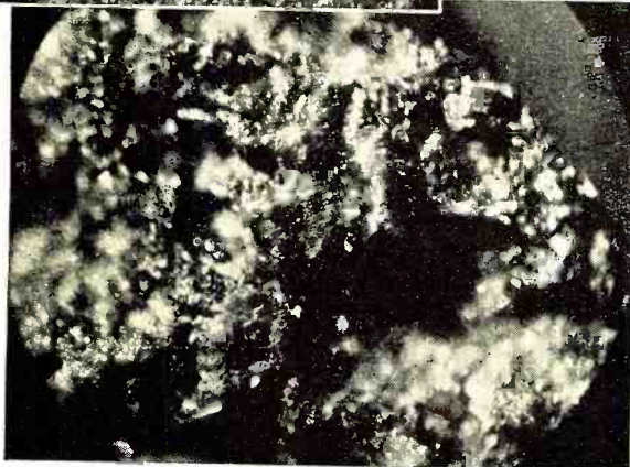
Ordinary resistor under 30-power microscope (unretouched photo) . . . Note rough surface which causes excessive heating;—gradual change in resistance.
