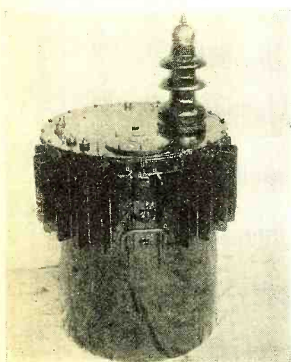
Figure 6. In this equipment, made by Waite and Bartlett Mfg. Co., the rectifier tube is operated in an oil bath
