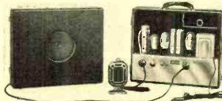
TYPE PG-63—A smaller and lighter design including close talking carbon microphone, Class B 6 watt amplifier and dynamic loudspeaker,—all self-contained in one convenient carrying case. Operates on 110 volt AC and is designed to reinforce speech and music, and has provision for electric phonograph input.
